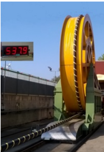
Figure 3 – examples of full-scale testing of submarine cable deep waters (source: paper Jicable 2019-A5.6) and for dynamic applications (source: paper Jicable 2019-C8.3)
