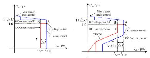
Figure 3 - Basic control characteristic Figure 4 - Optimized control characteristic
