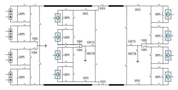
Figure 1 - Single diagram of Wudongde UHVDC
