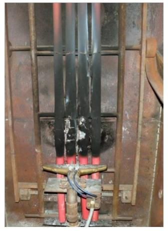
Figure 2 – Fire test according to IEC 60332-3 (source TB 720)
