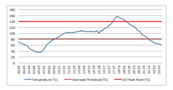
Figure 5 - Temperature Profile of an Overloaded PMT including the Overload Threshold and the Oil Flash Point
