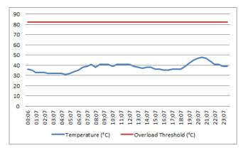
Figure 4 - Temperature profile of a loaded PMT
