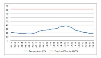
Figure 3 - Temperature profile of under-loaded PMT
