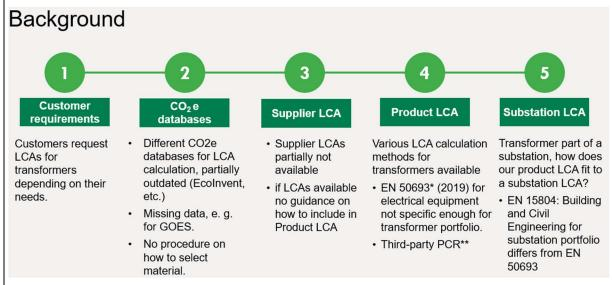
Figure 1. Background problem statement of Transformer LCA
